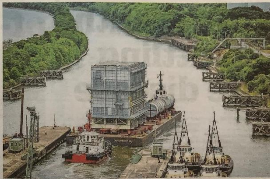
● The module has already been moved across the River Mersey and up the Manchester Ship Canal to a landing site next to the M53 in readiness for next week's three-mile move by road to Stanlow
